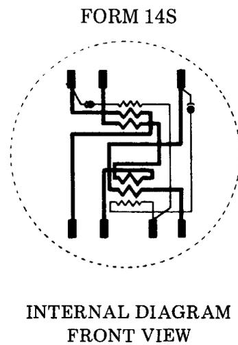
Measurement of energy on a three-phase, four-wire Wye service with a 3-stator meter.
