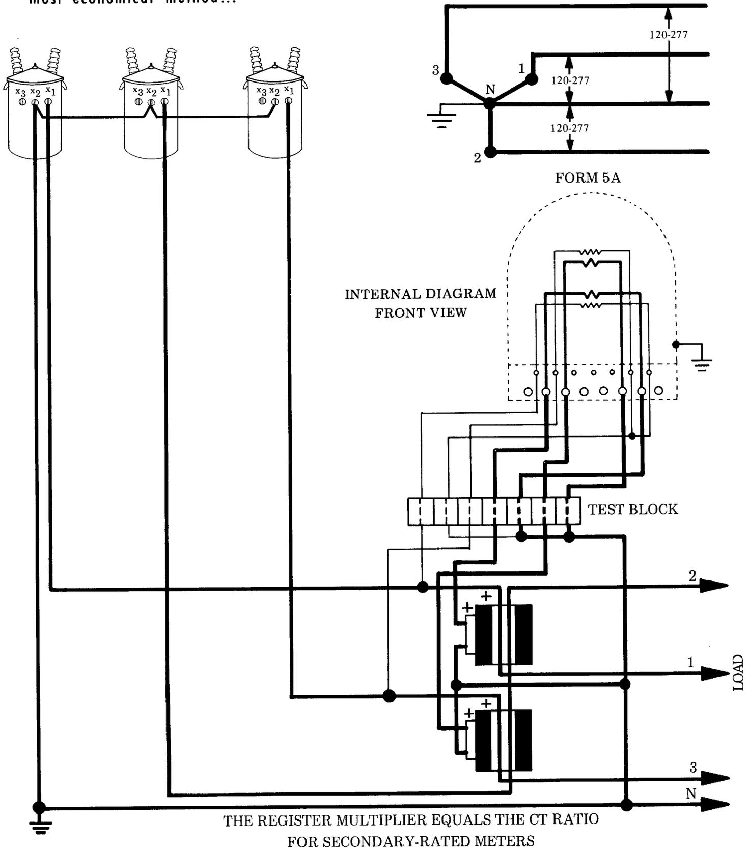
Measurement of energy on a three-phase, four-wire Wye service with 3 CT's (Delta connected secondaries), 2 VT's and a 2-stator meter.
