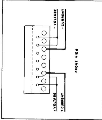
D5A-8, D4A-8, E1A-8E 3-phase, 4-wire, wye transformer-type — Right Stator Test. FORM 6A
