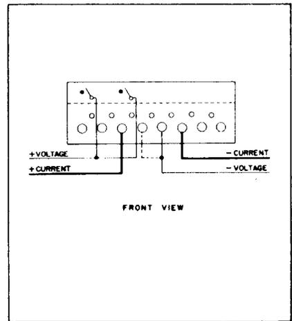
D5A-8, D4A-8 3-phase, 4-wire, wye self-contained — Right Stator Test. FORM 14A
