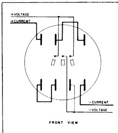
D5S-7, D4S-7, E1S-7E 3-phase, 4-wire, delta self-contained — Combined Stator Test. FORM 15S
