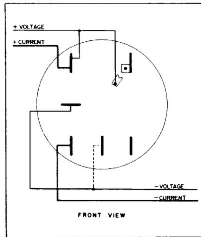
D5S-5, E1S-5E 1-, 2-, or 3-phase 3-wire, self contained — left Stator Test. FORM 12S
