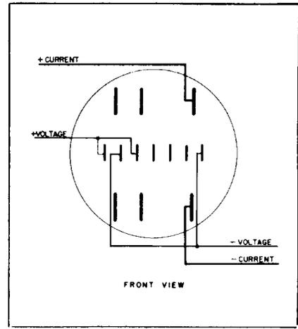
D5S-7, D4S-7, E1S-7E 3-phase, 4-wire, delta transformer-type – Right Stator Test. FORM 8S
