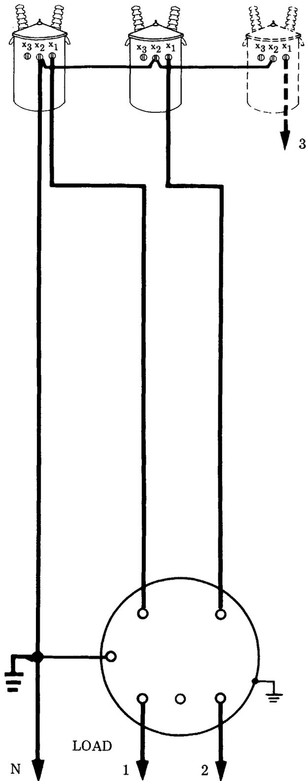
5-TERMINAL NON-CIRCUIT CLOSING SOCKET
