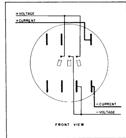
D5S-7, D4S-7, E1S-7E 3-phase, 4-wire, delta self-contained — Right Stator Test. FORM 15S
