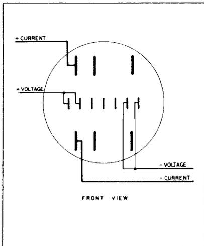
D5S-8, D4S-8, E1S-8E 3-phase, 4-wire, wye transformer type – Left Stator Test. FORM 6S
