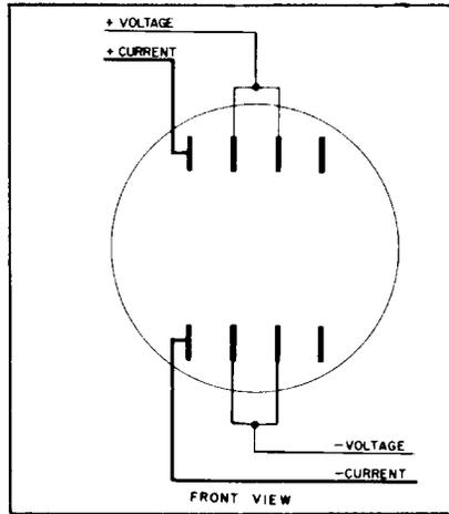
D5S-2, D4S-2, E1S-2E 1-, 2-, or 3-phase, 3-wire, self-contained and transformer-type — Left Stator Test. FORM 5S
