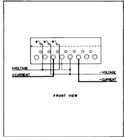
D5A-7, D4A-7 3-phase, 4-wire, delta self-contained — Right Stator Test. FORM 15A
