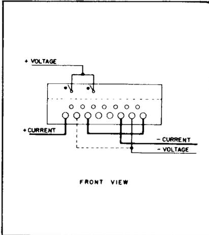
D5A-2, D4A-2 1-, 2-, or 3-phase, 3-wire, self-contained — Combined Stator Test. FORM 13A
