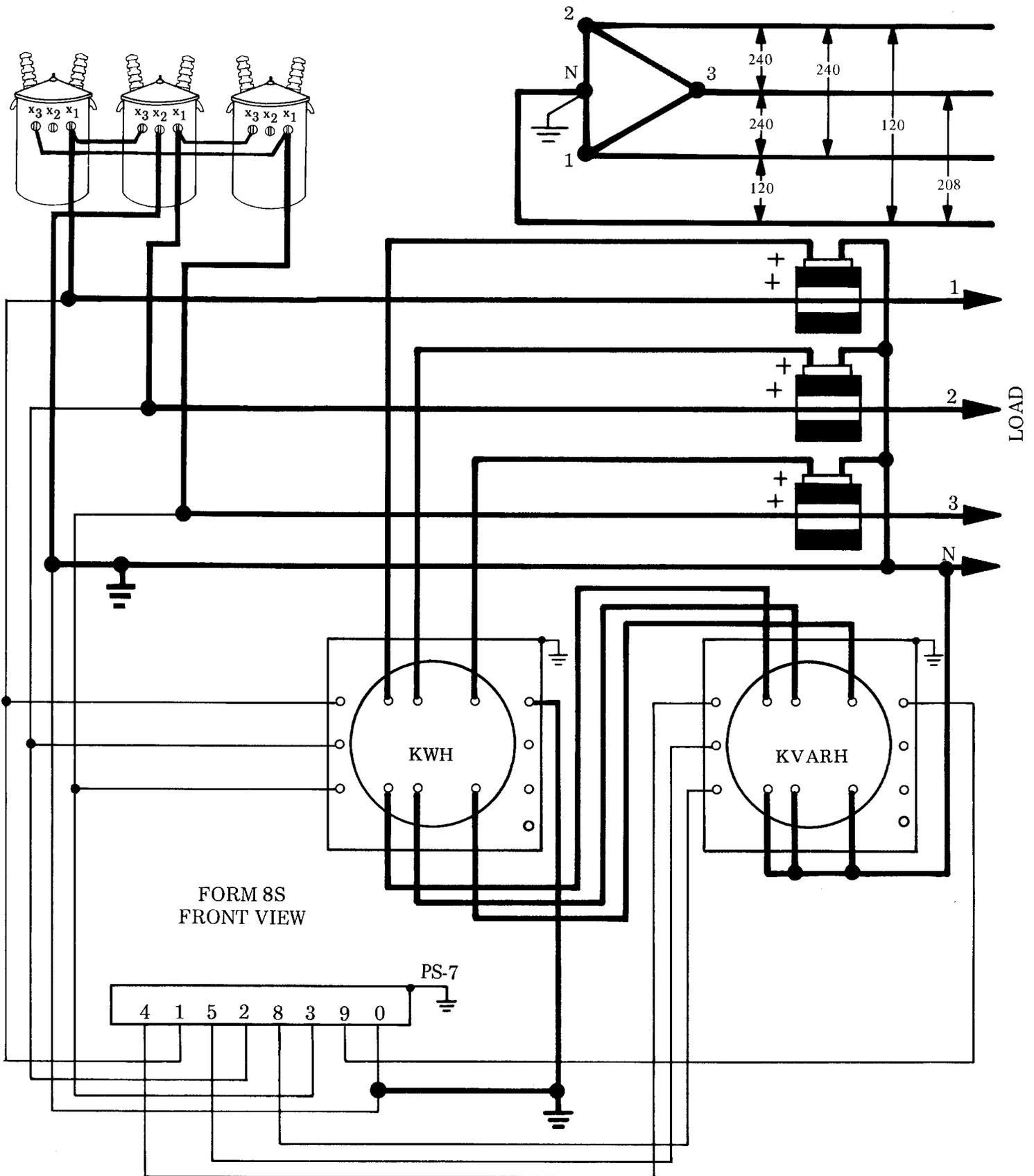
Measurement of KWH (and KW if required) and KVARH on a three-phase, four-wire Wye service with 3 CT's, 2 VT's, a phase-shifting transformer, and two 2-stator meters.
