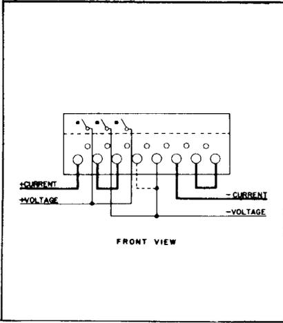
D5A-7, D4A-7 3-phase, 4-wire, delta self-contained — Combined Stator Test. FORM 15A
