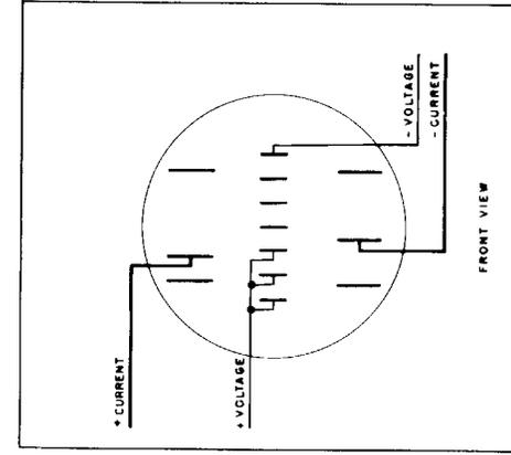
D5S-3, D4S-3, E1S-3E 3-phase, 4-wire, wye Tx Type — Rear Stator Test. FORM 9S
