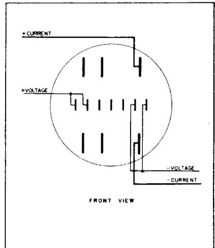
D5S-8, D4S-8, E1S-8E 3-phase, 4-wire, wye transformer-type – Right Stator Test. FORM 6S
