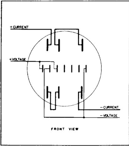
D5S-7, D4S-7, E1S-7E 3-phase, 4-wire, delta transformer-type – Combined Stator Test. FORM 8S
