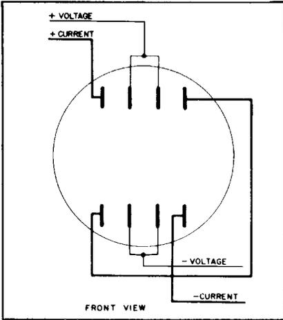
D5S-2, D4S-2, E1S-2E 1-, 2-, or 3-phase, 3-wire, self-contained and transformer-type — Combined Stator Test. FORM 5S
