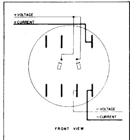
D5S-8, D4S-8, E1S-8E 3-phase, 4-wire, wye self-contained – Right Stator Test. FORM 14S
