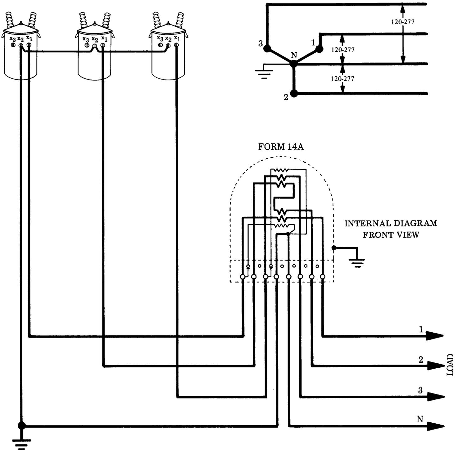
Measurement of energy on a three-phase, four-wire Wye service with a 3-stator meter.
