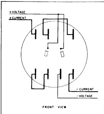
D5S-8, D4S-8, E1S-8E 3-phase, 4-wire, wye self-contained – Combined Stator Test. FORM 14S
