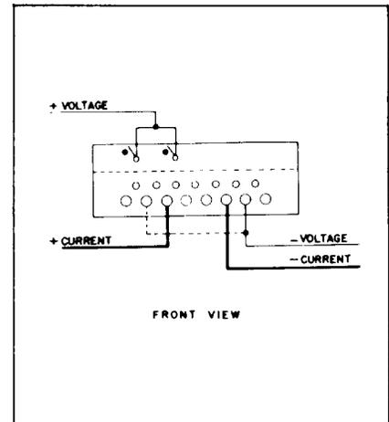
D5A-2, D4A-2 1-, 2-, or 3-phase, 3-wire, self-contained — Right Stator Test. FORM 13A
