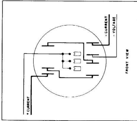
D5S-3, D4S-3, E1S-3E 3-phase, 4-wire wye self-contained — Combined Stator Test. FORM 16S
