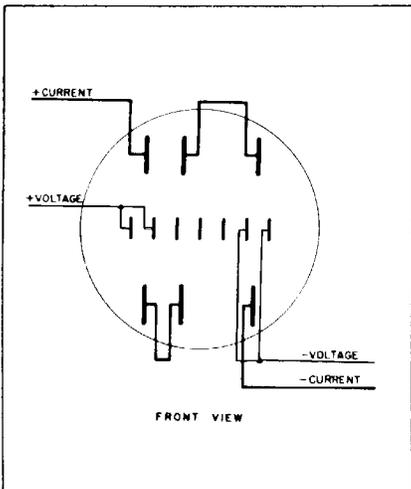
D5S-8, D4S-8, E1S-8E 3-phase, 4-wire, wye transformer-type – Combined Stator Test. FORM 6S
