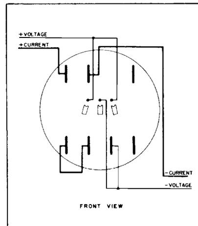
D5S-7, D4S-7, E1S-7E 3-phase, 4-wire, delta self-contained — Left Stator Test. FORM 15S
